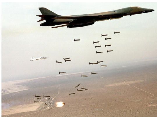
A B-1B Lancer unleashes cluster munitions. The B-1B uses radar and inertial navigation equipment enabling aircrews to globally navigate, update mission profiles and target coordinates in-flight, and precision bomb without the need for ground-based navigation aids.
